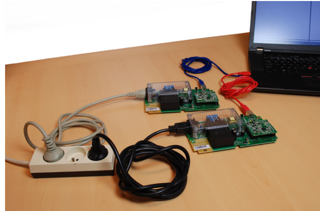
Figure 26. Connecting Both Modems to Single Distribution Strip Reduces the Noise Levels and Attenuation
