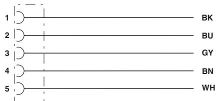
Contact assignment of 7/8" socket
