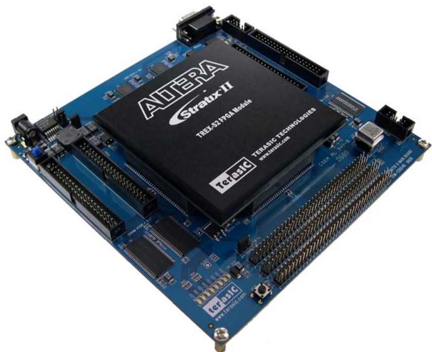
Figure 1.6 Terasic TREX-S2 Module with TREX-S2_TMB Motherboard
