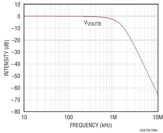
Figure 6. LT1568 Fourth Order Bessel Lowpass Filter (Linear Passband Phase)
