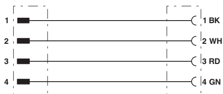
Contact assignment of 7/8" plugs/sockets
