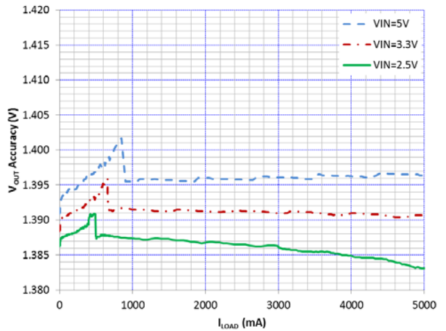
Figure 21. V_{OUT} Accuracy vs I_{LOAD} and V_{IN} , V_{OUT} = 1.394 V
