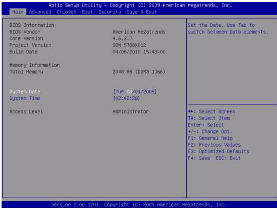
Figure 3.2 Main setup screen
