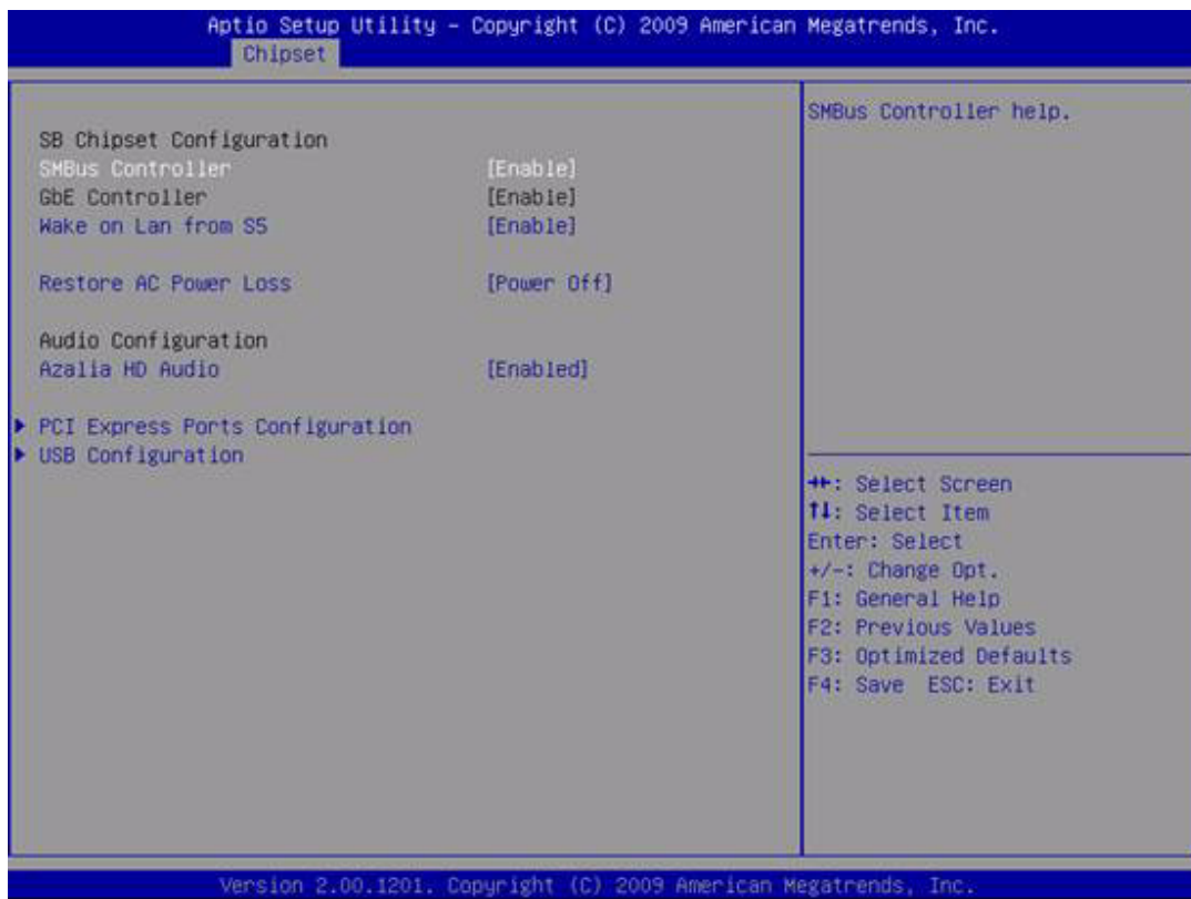
Figure 3.15 Chipset South Bridge Configuration
