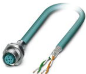
Bus system flush-type socket, Ethernet, 4-pos., M12, shielded, D-coded, SPEEDCON, rear/screw mounting with Pg9 thread, can be positioned, with 0.5 m bus cable, 2 x 2 x 0.2 mm 2
