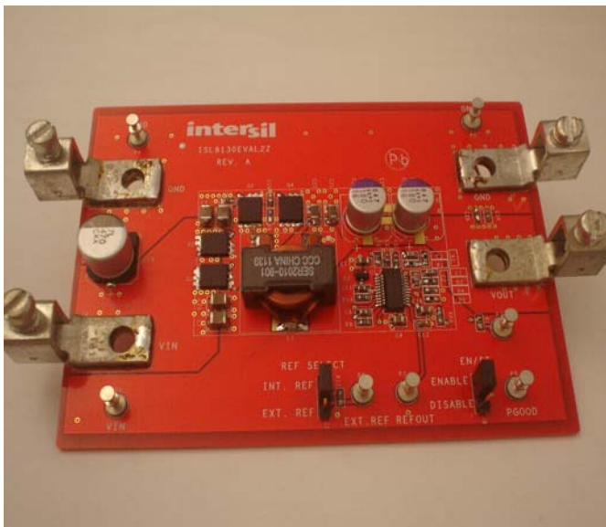
FIGURE 1. PHOTOGRAPH OF THE ISL8130EVAL2Z EVALUATION BOARD
