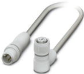
Sensor/Actuator cable, 4-position, PP-EPDM halogen-free, Gray RAL 7035, Plug straight M12, A-coded, on Socket angled M12, A-coded, Cable length: 0.6 m, Hygienic design, with plastic knurl
