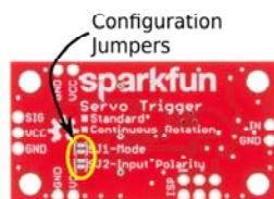
Configuration Jumpers, SJ1 and SJ2.
