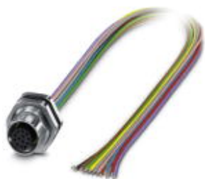
Flush-type connector, Universal, 8-position, Socket, Link: M12, A-coded, Rear mounting, M16 x 1.5, Individual wires, Cable length: 0.5 m
