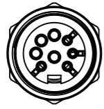
AISG 8-pin female interface with 4 loaded contacts
