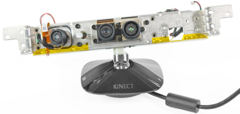
Figure 1-1. A Kinect with its plastic casing removed, revealing (from left to right) its IR projector, RGB camera, and IR camera. (Photo courtesy of iFixit.)
