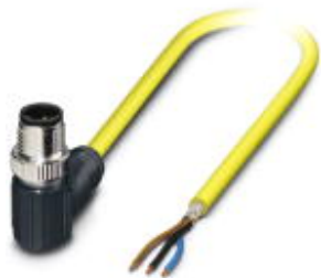
Sensor/Actuator cable, 3-position, PVC, yellow, shielded, Plug angled M12 SPEEDCON, A-coded, on free cable end, Cable length: 5 m
