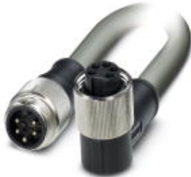
Bus system cable, DeviceNet, 5-position, PVC, Gray RAL 7001, Plug straight 7/8"-16UNF, on Socket angled 7/8"-16UNF, Cable length: 1 m
