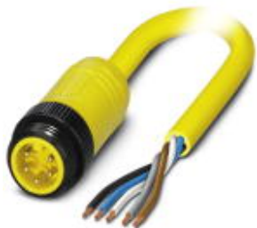
Power cable, 5-position, PVC, yellow, Plug straight 7/8"-16UNF, A - standard, on free cable end, cable length: 1 m
