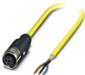
Sensor/Actuator cable, 3-position, PVC, yellow, shielded, free cable end, on Socket straight M12 SPEEDCON, A-coded, Cable length: 2 m
