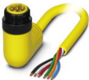
Power cable, 6-position, PVC, yellow, Plug angled 7/8"-16UNF, on free cable end, cable length: 1 m
